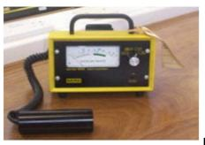
A modern Geiger Counter is at left, and the way the device works is shown in blue. The gas atoms are ionized and "counted" by the high voltage wire strung through the center.
